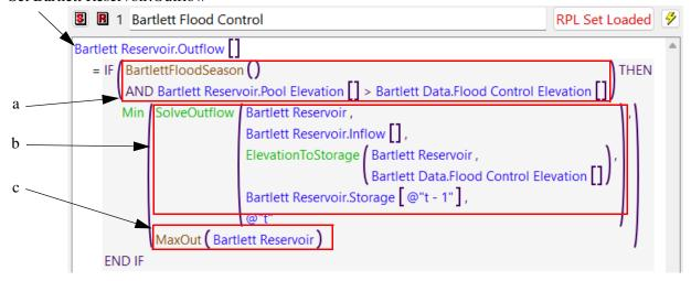
The rule contains logic (IF, THEN), slot names (e.g. Bartlett.Pool Elevation), and functions, both user defined and predefined functions. In general, it says:
