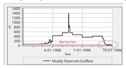
Looking at the right side of the Muddy Outflows plot, we see that the Min Fish Flow is not being met at the end of the simulation period either. It appears that there could be another problem with either the policy or the date. We can use the RPL Debugger to find out why the minimum flow is not being met.
