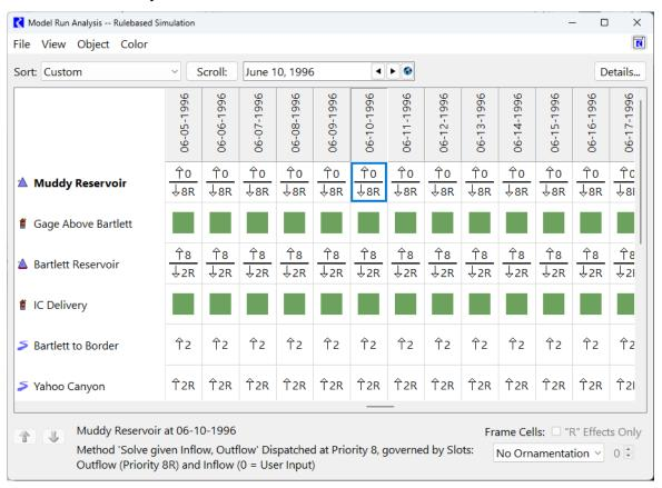
Scroll through the timesteps horizontally and notice the reservoirs and reaches were dispatched in accordance with various rules in the model ruleset.
