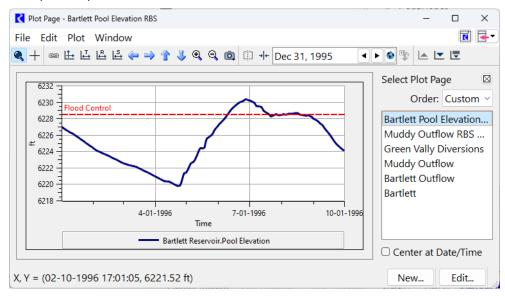
If you remember, we saw that the Flood Control rule is turned off. Therefore there is no logic or policy in effect to keep the Bartlett Pool Elevation from exceeding maximum prescribed elevation. We see this illustrated in the plot in July 1996. In the next section, we'll turn on the rule and see its effect.
