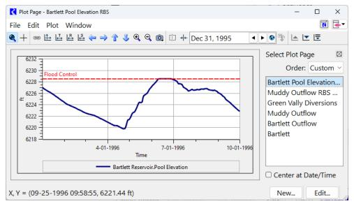
Now that the **BartlettFloodControl** rule is activated, Pool Elevation does not exceed the Flood Control height at any time. Because the rule has the highest priority, no other operation request (i.e. rule) can override it.
