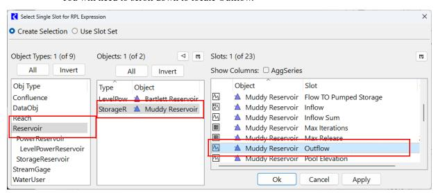
You have finished the left-hand side (LHS) of the rule. When the rule is executed, the rulewill attempt to set a value on the Muddy Reservoir Outflow slot to the value returned from the right-hand side (RHS) of the assignment.
