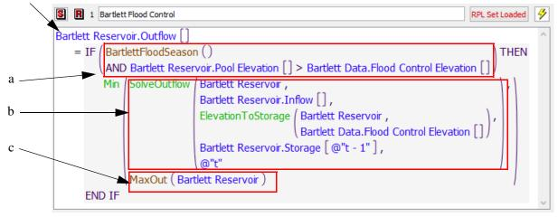
The rule contains logic (IF, THEN), slot names (e.g. Bartlett.Pool Elevation), and functions, both user defined and predefined functions. In general, it says:
